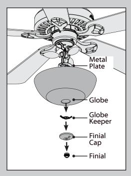
Changing the bulbs - unscrew the finial and remove it from the threaded rod. Remove the finial cap and unscrew the globe keeper while supporting the globe with your other hand. Carefully remove the globe. Unscrew bulbs and replace with bulbs of same type and wattage. Reinstall the globe assembly.
